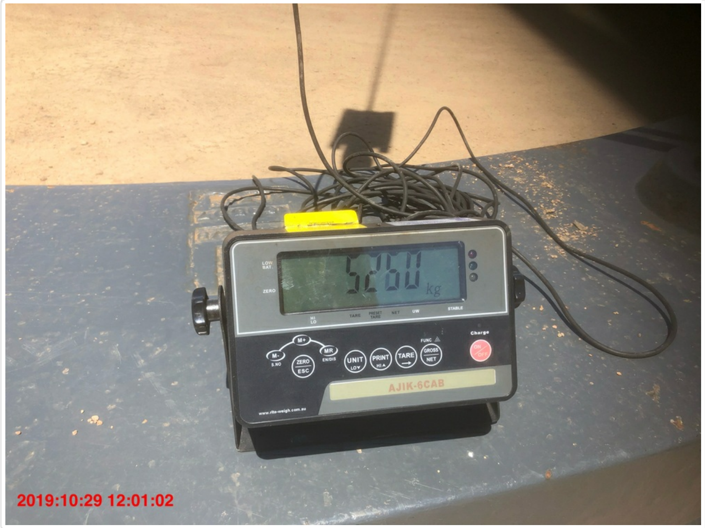
Rated Load - Boom Fully Extended - Load Measured
