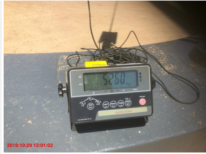
Rated Load - Boom Fully Extended - Load Measured
