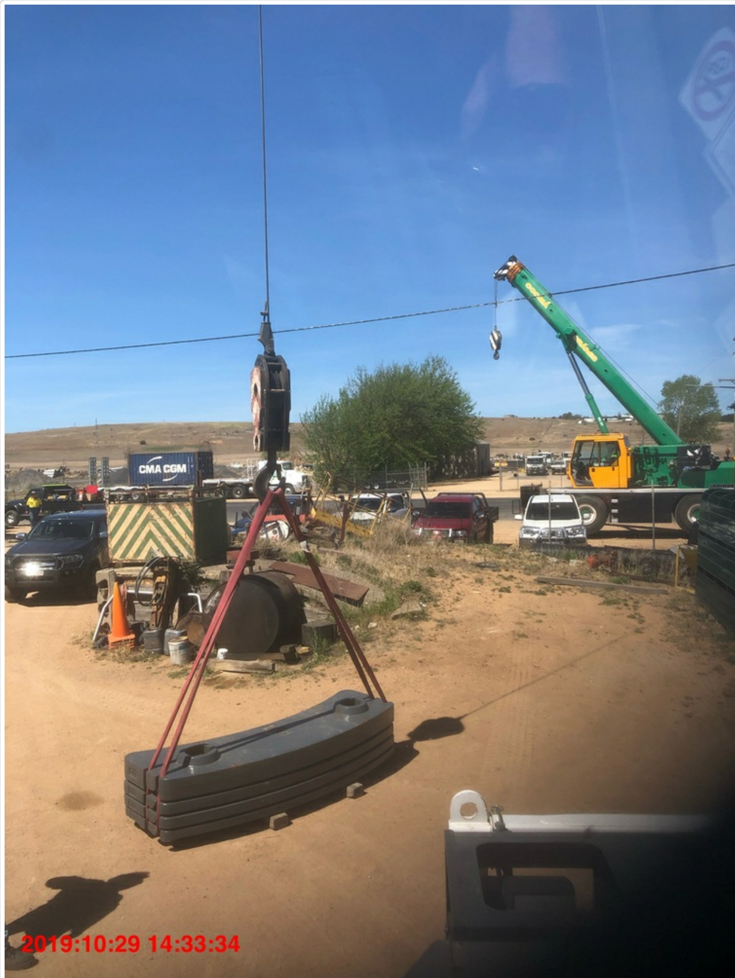
Line Pull Test - Load Measured
