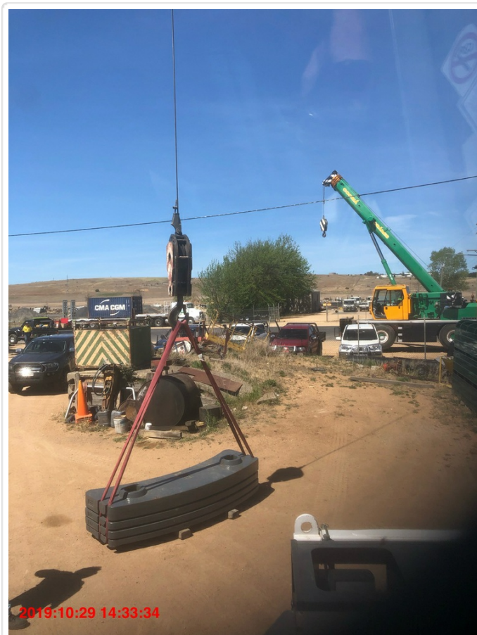
Line Pull Test - Load Measured
