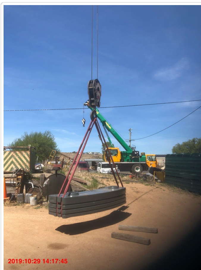
Rated Load - Boom Fully Extended - Load Measured
